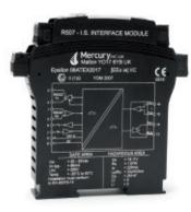
Connection to a Mercury Terminal in the Hazardous Area is by a simple Quad core or two pair cable, carrying power and full duplex serial data together with multi-drop control at up to 1km distance.
